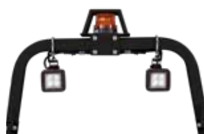
STROBE & WORK LIGHTS Provides increased safety for roadside operation and low-visibility situations. (comes in two separate kits)
