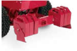
2-N-1 Allows for the option of a front 2-inch receiver hitch or front counterweights.
