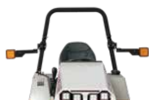
DIRECTIONAL HAZARDS Directional LED signals/ blinking hazards.
