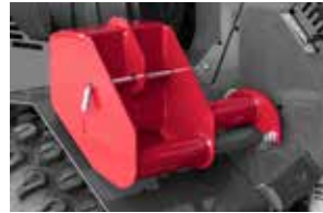
MID-WEIGHT BAR KIT Add up to four additional weights to the middle of your 4000 series Ventrac
