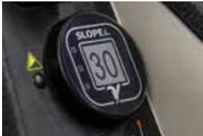
DIGITAL SLOPE INDICATOR Indicates the degree of slope while tractor is in operation.
