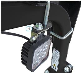
**Note:** If the mounting stud on the work light does not fit in the mounting hole in the canopy mount plate<sup>①</sup>, either drill the hole to fit the light stud or replace the canopy mount plates with the mount plates from the original rear work light kit.
