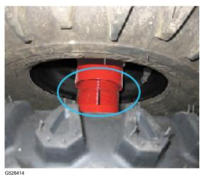
14. If the steering cylinder is mounted to the inner hole setting of the steering cylinder mount, move the steering cylinder to the center hole setting of the cylinder mount under the left front corner of the foot platform. Torque to 203 N·m (150 ft-lb).
