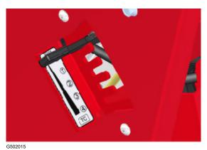
To set the weight transfer, raise the front hitch to its maximum height and move the weight transfer select lever to the desired position.
