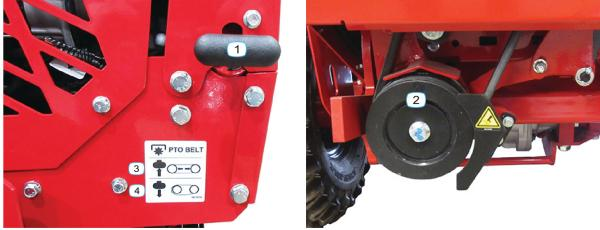
The PTO belt tensioner rod<sup>1</sup> applies or releases belt tension to the attachment drive belt. After placing the attachment drive belt onto the PTO drive pulley<sup>2</sup>, push the PTO belt tensioner rod in<sup>3</sup> until it locks in position with tension applied to the attachment drive belt. Pulling the PTO belt tensioner rod out<sup>4</sup> releases the belt tension, allowing the operator to remove or install the attachment drive belt.
