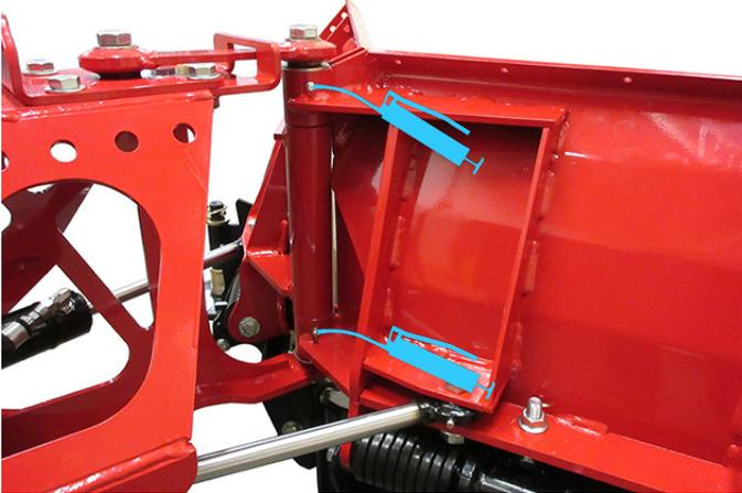
Adjust the blade wings to the swept back position and detach the V-blade from the power unit. Grease the wing blade cylinder ends.
