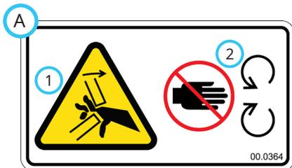
1. Pinching or crushing hazard.
