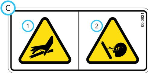
1. High pressure fluid hazard - keep your body and hands away from suspected hydraulic leaks.
