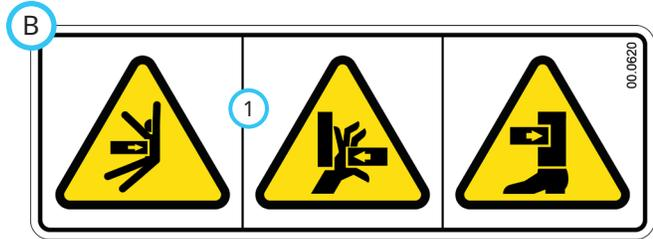
1. Pinching or crushing hazard.
