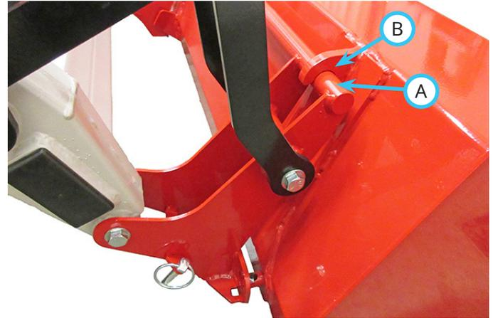
4. Tilt the tool mount frame back until the latch pins protrude through the lower latch plate on the tool mount frame.
