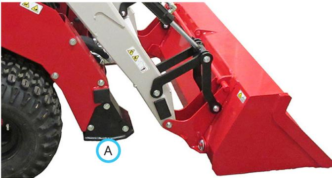
6. Lower the loader arms until the bucket or tool is resting on the ground.
