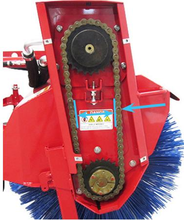
4. If the chain tension needs adjusted, refer to the following section for adjustment procedures. If chain tension is correct, reinstall the drive chain cover and torque the bolts to 8 Nm (67 in-lbs).
