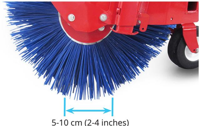
6. If the distance falls outside the suggested measurement, raise the broom to the highest position and support the broom frame with blocks or jack stands.
