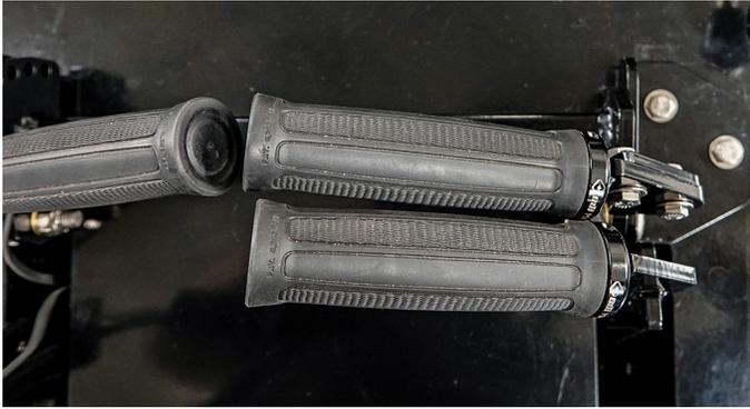
17. Tighten the hardware that fastens the right drive control handle to the right control arm. Torque to 24 N·m (210 in-lbs).
