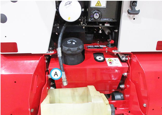
7. Remove the drain cap from the drain hose and drain the engine oil into the pan while the oil is warm.
