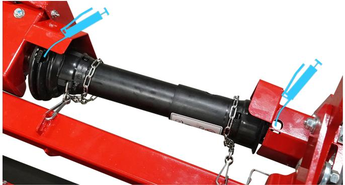
Rotate the drive shaft covers until the access holes align with the grease fitting on the drive shaft slide.
