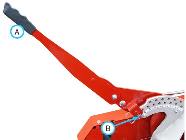
2. Pull back slightly on the handle to relieve pressure on the locking pin and remove the locking pin (B) from the rear carrier rocker.
