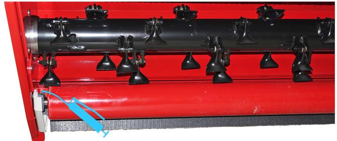
Grease the left rear roller bearing.
