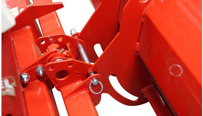
8. To return the deck to the operating position, remove the pin from the cross frame brackets and lower the deck to the operating position. NOTE: if the front hitch lowers due to hydraulic drift, it may be necessary to start the power unit's engine and raise the front hitch before removing the pin.
