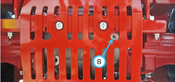
3. Remove the drain plug (B) from the rear transaxle and allow the hydraulic oil to drain. Remove the oil fill plug (C) from the rear transaxle to allow venting.
