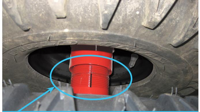
After tightening the outer dual wheel, there should be four or fewer threads visible on the outer dual wheel extension.
