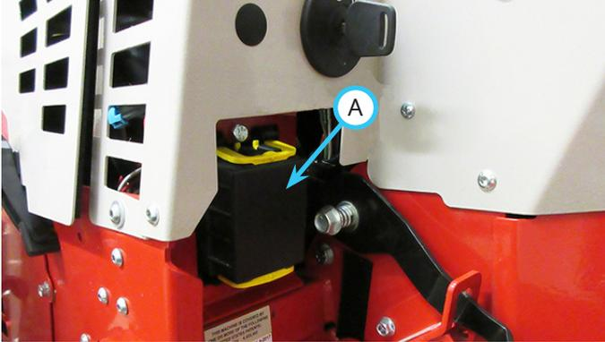
3. Identify and remove the defective fuse from the socket. Refer to the Quick Reference decal under the hood for fuse locations.
