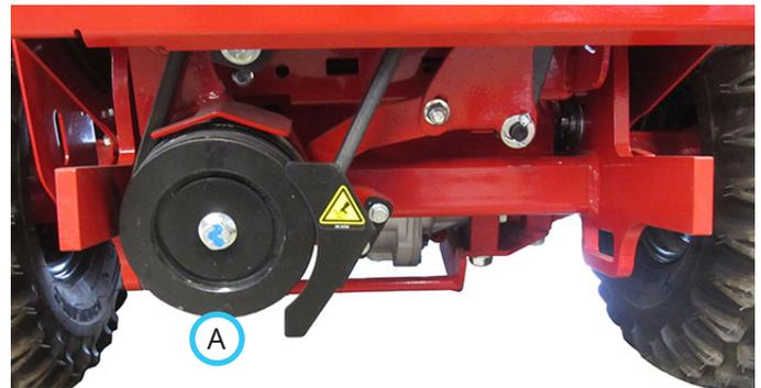
When the belt is in place around the drive pulley, push the PTO belt tensioner rod in to engage and tighten the belt.
