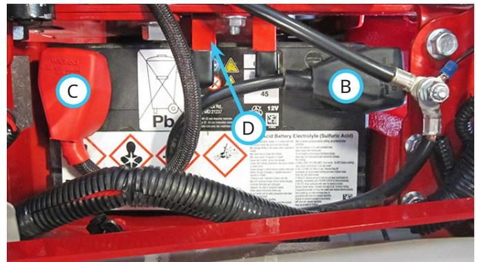
5. Remove the battery retainer (D).
