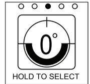
**Display Screen 4** displays the total slope angle in degrees, along with independent front-to-back angle and side-to-side angle.
