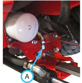
6. Remove the drain cap from the oil drain and drain into the pan while the oil is warm.
