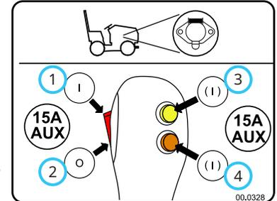
Press the top (1) of the rocker switch to turn on the electrical power to the 4-pin socket. Press the bottom (2) of the rocker switch to turn off the electrical power.
