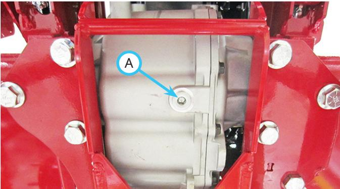
7. Reinstall the plug into the front transaxle and torque to 34-39 Nm (25-29 ft-lbs).
