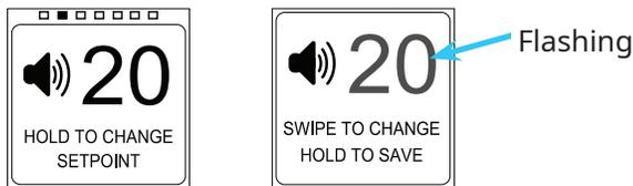
When the desired set-point is reached, hold over the sensor to save the setting.
