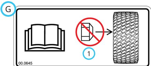
1. Place this side of the rim against the axle hub. Do not install the wheel lug nuts on this side of the rim. Refer to the operator's manual.
