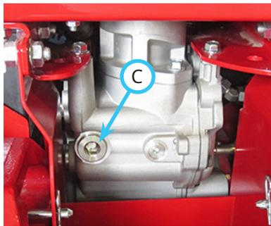
NOTE: on some power units, it may be necessary to remove the rear transaxle skid plate to access the drain plug.
