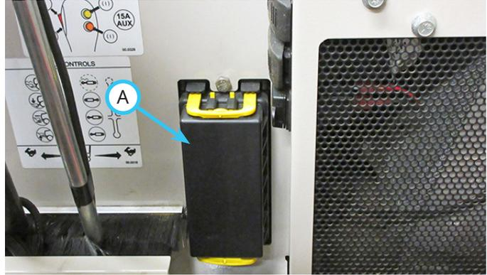
4. Identify and remove the defective fuse from the socket. Refer to the Quick Reference decal under the hood for fuse locations.
