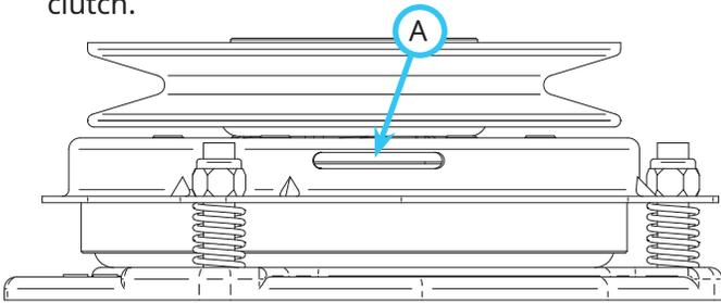
2. Insert a .5 mm (.020 inch) feeler gauge through the inspection window and into the slot between the armature and the rotor.
