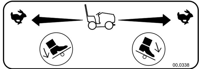
The foot pedal works in conjunction with the SDLA control lever and can be used to control the speed and direction of the power unit when the operator's hand is removed from the SDLA lever.
