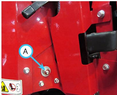
9. Loosen the neutral adjustment nut (A) slightly. NOTE: it is easier to attain the desired setting if the neutral adjustment nut is left snug and a rubber mallet or a piece of wood and a hammer are used to tap the nut in the desired direction. Do not strike the nut directly with a metal hammer, as it is possible to dent or damage the nut.
