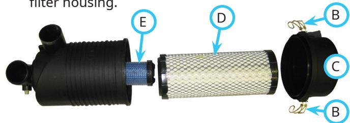
3. Remove the filter cap (C).
