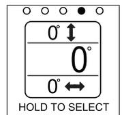
**Display Screen 5** displays the total slope angle in degrees, along with independent front-to-back angle and side-to-side angle with position indicators.
