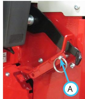
Ensure the shift lever is secured in the lock position at the end of the shift stroke. Reinstall the ball pin (A) into the shift select bracket position at the same end as the shift lever, in order to prevent the shift lever from being accidentally disengaged.
