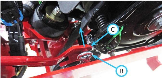
6. Remove the belt tensioner rod from the belt tensioner rocker.
