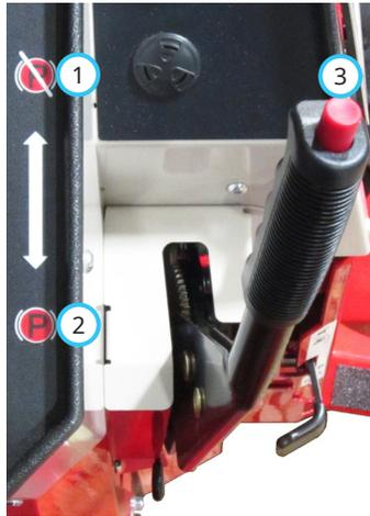
1. Parking Brake Disengaged
