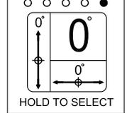
When the desired screen is reached, hold over the sensor to select and save. The slope gauge will remember the selected screen when the power unit is shut off and will display the selected screen when the power unit is restarted.
