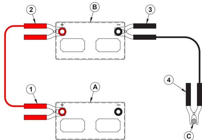
A. Discharged Battery      C. Ground Stud
