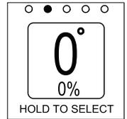
**Display Screen 3** displays the total slope angle in degrees, along with a visual horizon and roll indicator.
