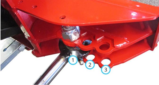
1. **Standard position:** this position is the standard position and enables the tightest turning radius.
