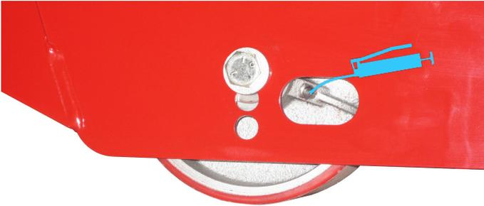
2. Grease the caster wheel axles and pivots.
