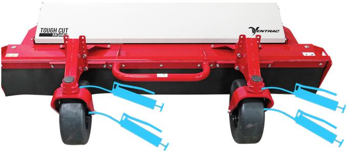
3. Grease the drive shaft bearings.
