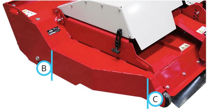
9. To lower the rear of the mower deck, move the hitch arm pins to a higher position. To raise the rear of the mower deck, move the hitch arm pins to a lower position.
