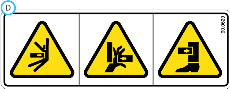
Pinching or crushing hazard.
