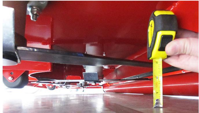
7. Rotate the blade so the same tip is at the front of the deck and measure again. The blade tip should be level to 3 mm (1/8 inch) lower at the front. If the measurement at the front is greater than at the rear or is more than 3 mm (1/8 inch) lower than at the rear, the deck must be leveled.
