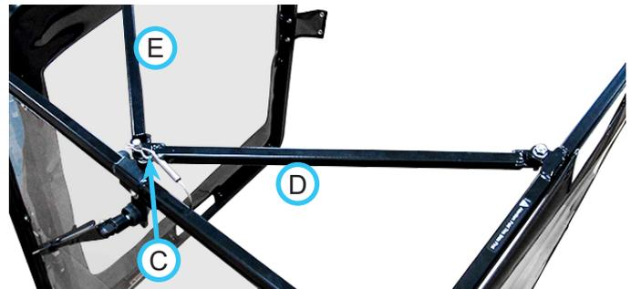
8. Lift the right crossbar (E) off the pin, rotate to the rear of the windscreen, and place in its retaining bracket.
