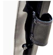
26. Unfold the front of the left canvas and make sure the internal magnets hold it securely to the front frame.
