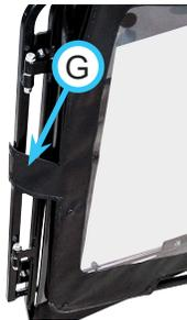
22. Remove the windscreen from the box, unsnap the retaining flap (G), and unfold the windscreen sides.
