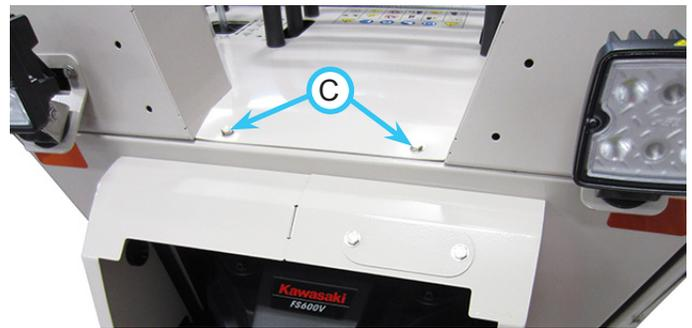
11. Power units with serial numbers 01001 - 01230 will require mounting holes to be drilled in the outer dash panels. For power units outside this range, skip to step 16.
