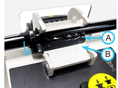
5. Slide the windscreen assembly back out of the mounting points on the front dash mount.
