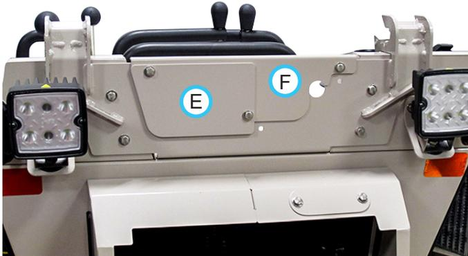
18. If the power unit is equipped with a brine system, discard the dash cover plate (E). Remove the pieces of rubber trim from the old front dash mount and front cover plate and install onto the new front dash mount and front cover plate.
