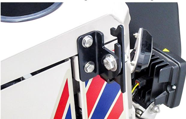
7. Adjust the rear post and door assembly until the door closes properly and aligns with the dash and front cover. Torque bolts to 67 in-lbs (8 Nm).
