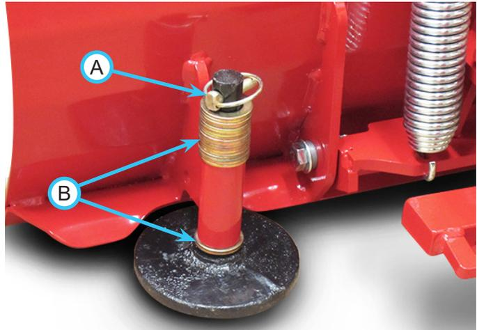
5. Remove the skid shoe from the bottom of the skid shoe mount. Add or remove spacer washers to reach the desired skid shoe height.
