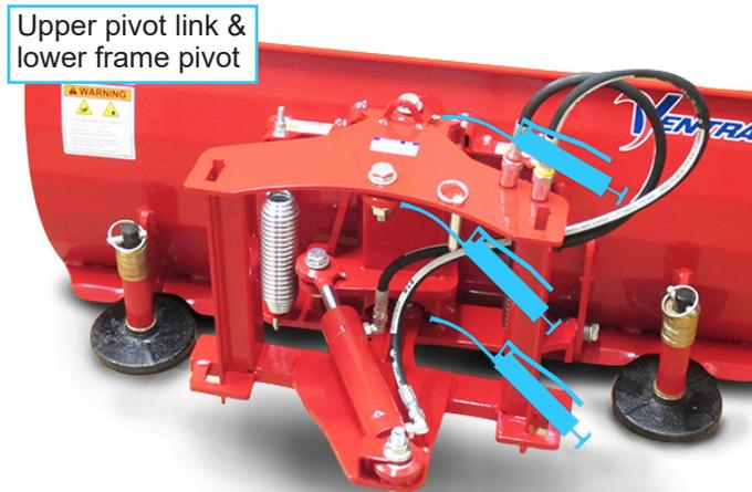
Angling the snow plow blade to the left helps increase access to the grease fitting in the lower frame pivot.
