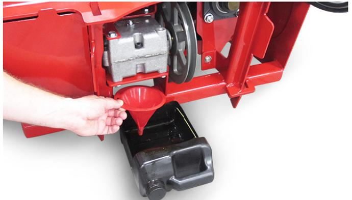
6. Remove the pipe plug from the bottom port of the gearbox and use the funnel to direct the gear oil into the drain pan.
