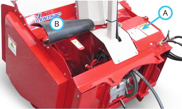
3. Flip open the belt adjustment cover belting (B).
