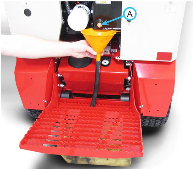
8. Remove the drain plug from the hydraulic oil tank and allow the hydraulic oil to drain from the system. Loosen the dipstick on the hydraulic oil tank to allow venting.
