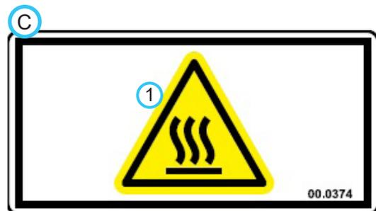
1. Hot surface hazard - Hot surfaces can cause severe burns. Allow engine, exhaust components, and surrounding surfaces to cool before servicing.
