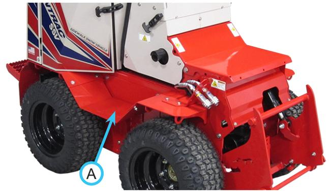
9. Use a 3/8" drive ratchet to rotate the PTO belt tension arm far enough to remove the belt from the belt tension pulley.
