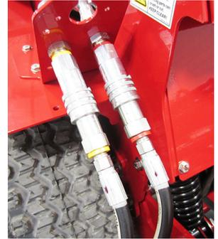
To disconnect the couplers, pull back on the collar on the power unit coupler to release the attachment hose.
