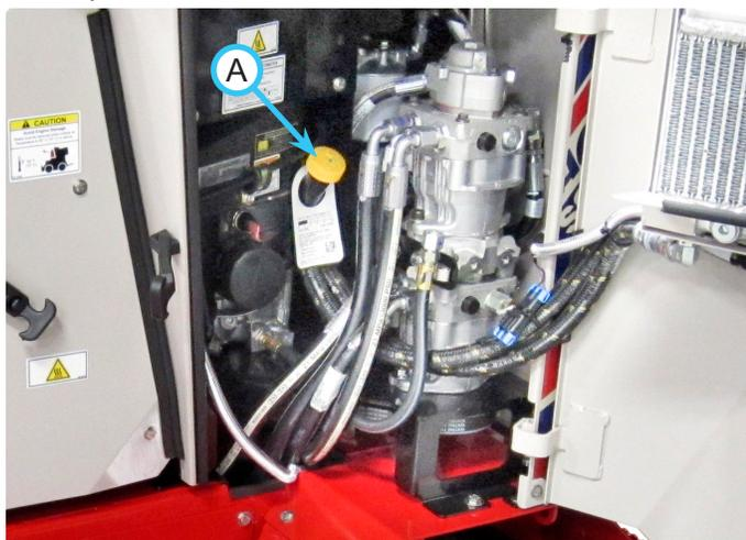
6. Insert the dipstick back into the engine without threading it in and remove again.
