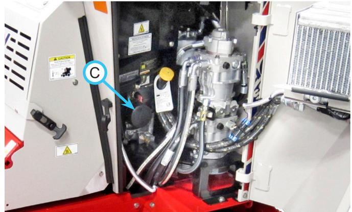
9. Wipe the filter mounting surface with a clean cloth.
