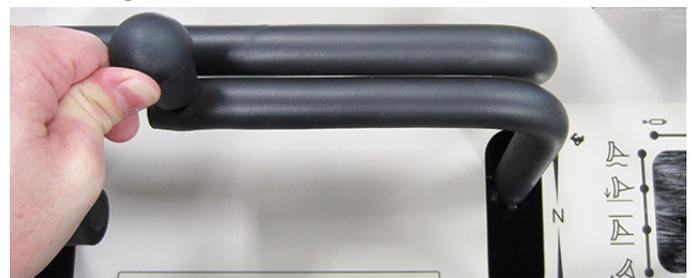
19. Tighten the hardware that fastens the right drive control handle to the right control arm. Torque to 210 in-lbs (24 Nm).
