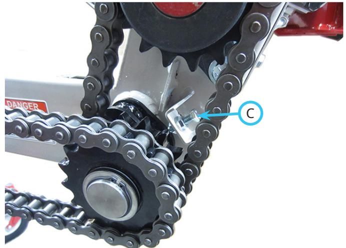
8. Tighten the locking nuts to secure the stop bolt.
