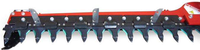
3. Position the clamps (C) on the drive link base and loosely install the bolts.
