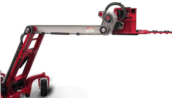
3. Rotate the main arm until the outer arm is parallel with the ground.
