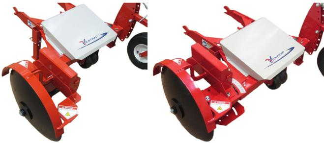
The edger disc can be positioned either in front of or behind the main frame receiver tube. NOTE: if the edger is equipped with an optional blower kit, positioning the disc behind the main frame receiver tube will block the airflow and prevent debris from being blown away from the edging location.
