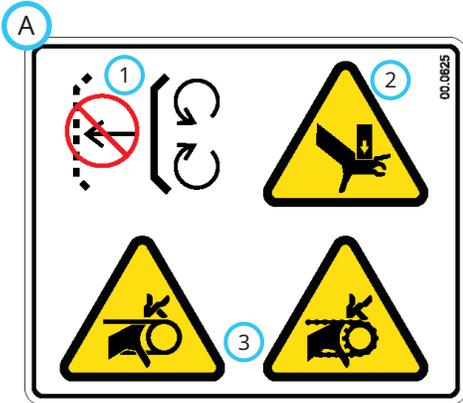
1. Shield missing - do not operate.
