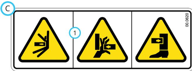
1. Pinching or crushing hazard.
