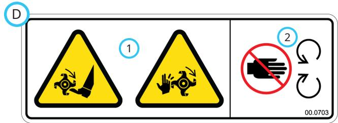
1. Cutting or dismemberment hazard of hand or foot - rotating tine.
