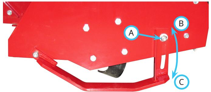
5. Check to make sure both the left and right skid shoes are set to the same position and tighten the adjustment bolts.
