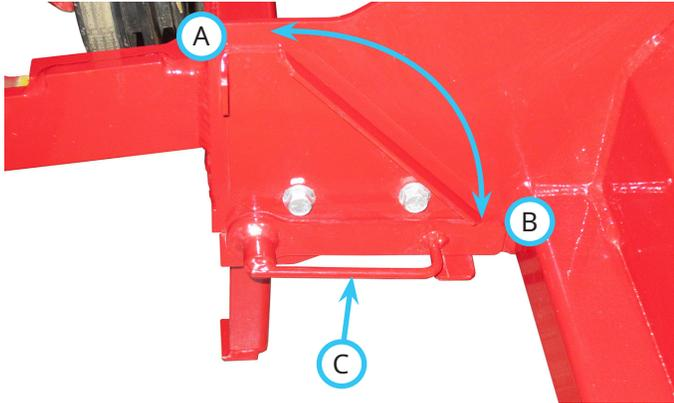
Place the jack stand in the storage position (B) prior to detaching from the power unit.
