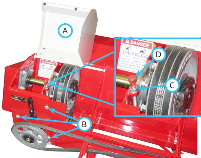
3. Remove the drive pulley shield from the tiller.
