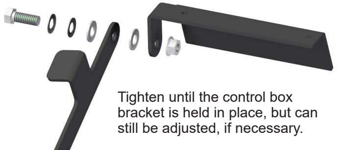
Tighten until the control box bracket is held in place, but can still be adjusted, if necessary.
