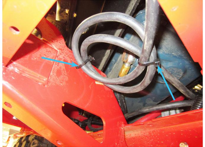
36. Use a zip tie to fasten the wire harnesses to the main wire harness in the rear frame behind the rear transaxle.
