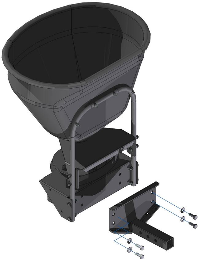
2. Slide the spreader hitch tube into the hitch receiver and fasten with the included 5/8 x 3" hitch pin. Use the hole in the spreader hitch tube that positions the spreader closest to the power unit without any contact between them.
