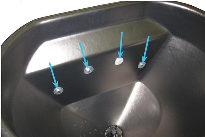
6. Place 1) 64.1686 vibrator mounting plate on the inside of the plastic hopper and the 2nd mounting plate on the outside of the plastic hopper.
