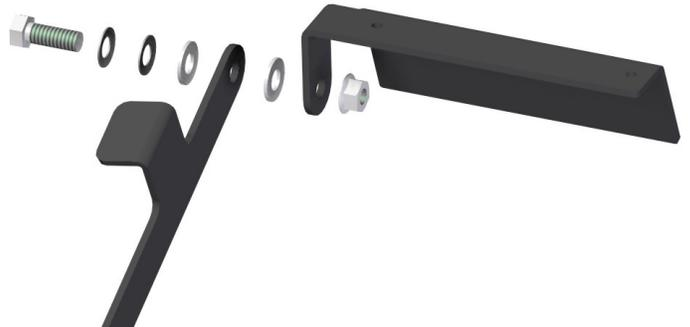
Tighten until the control box bracket is held in place, but can still be adjusted, if necessary.
