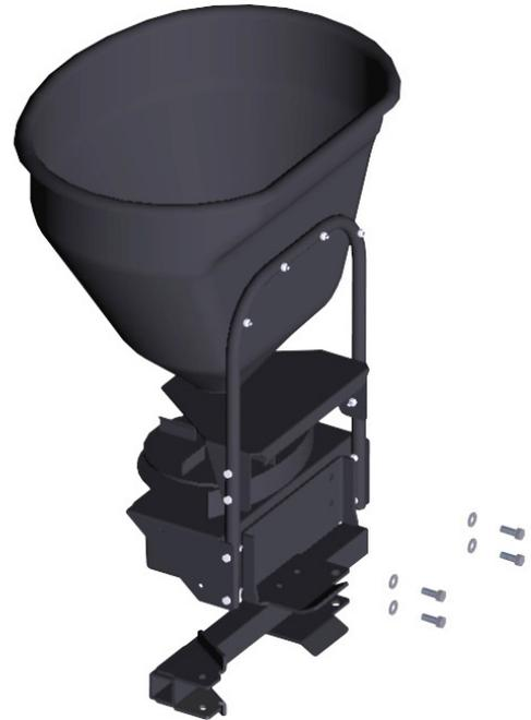
2. Install the spreader pivot hitch onto the tractor pivot hitch and align the holes in the spreader pivot plates with the hole in the tractor pivot tube. Place 2) 5/8" flat washers onto the 5/8" x 4-1/2" bolt and insert in the pivot plates and tube. Place 2) 5/8" flat washers onto the
