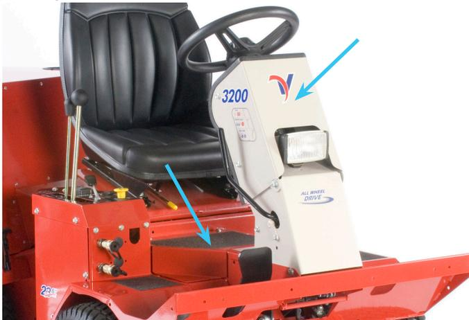
box mount bracket hooked over the top edge of the steering column cover. Do not tighten.
