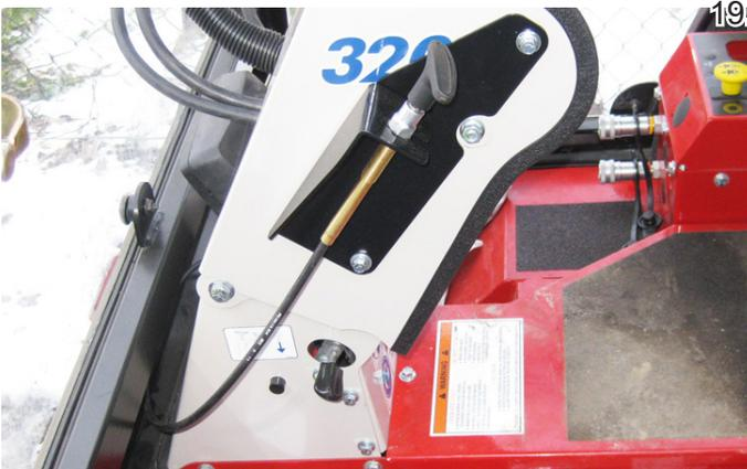
20. Remove the bolts that fasten the foot pedal pivot to the front frame. Install a supplied 1/4" x 3/4" bolt and clamp in the front hole of the foot pedal pivot on the top side of the front frame. Place the gate cable in the clamp and tighten the bolt.
