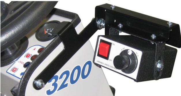
10. Connect the battery/controller harness to the battery lead on the controller.
