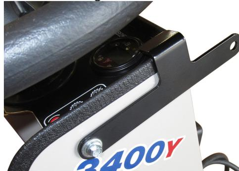
25. Place 2) disc springs onto a 3/8" x 1" bolt. Orient the disc springs so the peak of the coned disc is against the bolt head. Place a 3/8" flat washer onto the bolt and insert through the hole on the control box mount bracket as shown below. Place another 3/8" flat washer onto the bolt, install the control box bracket onto the bolt, and fasten with a 3/8" locking flange nut.
