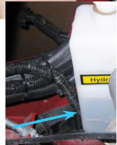
6. Route the harness over the top edge of the frame and down between the rear frame flange and the engine hood hinge bolt. Use a zip tie to fasten the motor/controller wire harness to the rear frame flange with the end of the motor/controller plug approximately 4" below the bottom of the frame.
