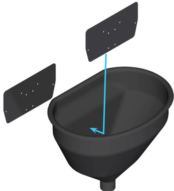
7. Use the hardware removed in step 5 to fasten the vibrator mounting plates and the hopper to the spreader frame. Torque to 135 in-lbs (15 Nm).
