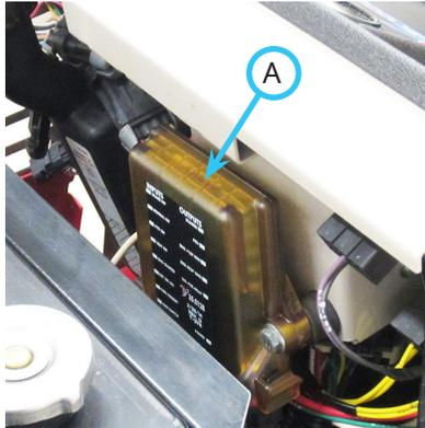
This TCM monitors the electronic circuits necessary for the engine, the starter, and the PTO to function. These input circuits include the PTO switch, the neutral switch, the parking brake switch, the ignition switch, the seat switch, and the generator presence. The TCM is programmed to allow the engine, the starter, or the PTO to operate only when specific input criteria are satisfied. The engine, the starter, and the PTO are controlled by outputs from the TCM.
