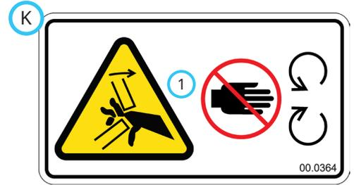
1. Cutting or pinching hazard. Stay away from moving parts.
