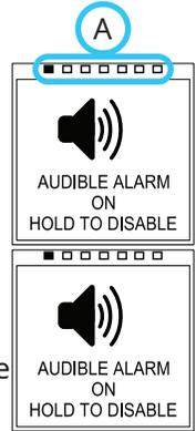
**Menu Screen 1** allows the user to mute or enable the audible alarm. The screen will display the current state of the alarm. Hold over the sensor for three seconds to change the setting.
