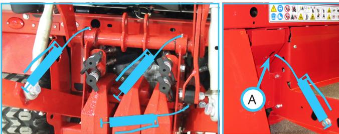
The front grease fitting on the 3 point cylinder can be greased through an access hole (A) in the right foot platform panel.
