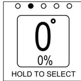
**Display Screen 3** displays the total slope angle in degrees, along with a visual horizon and roll indicator.
