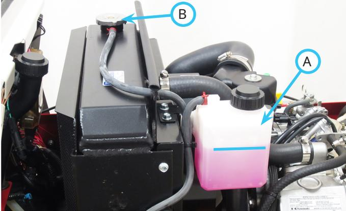
4. If the coolant level is low, add coolant to the tank and reinstall the cap.
