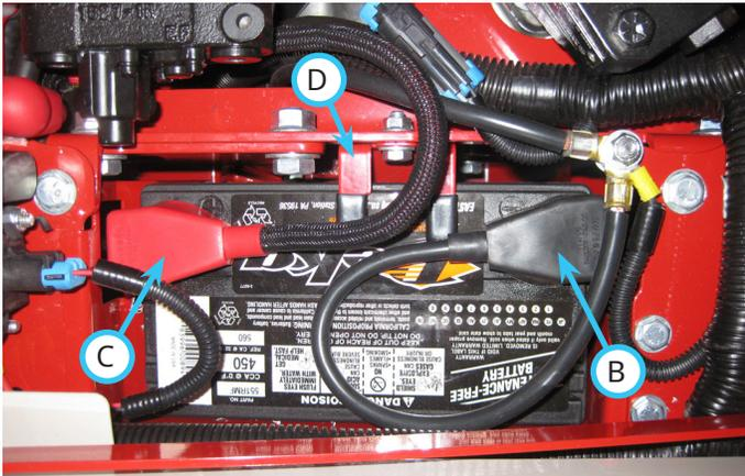
5. Remove the battery retainer (D).
