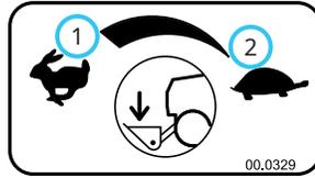
The front hitch and attachment can be locked in any position, so that it will not lower, by turning the front hitch valve knob clockwise until it is completely closed. When operating 3 point hitch implements, it may be helpful to lock the front hitch and attachment in a raised position, to prevent accidental lowering of the front attachment.
