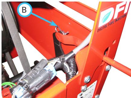
6. Remove the belt tensioner rod from the belt tensioner rocker.
