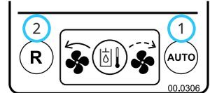
The switch can be set to the reverse position (2) to pull air from the rear of the power unit, through the oil cooler, and discharge the warm air next to the operator. This feature can be used to help provide warmth for the operator during cold weather.
