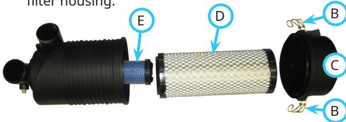
3. Remove the filter cap (C).
