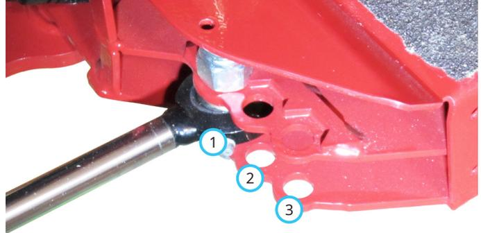
1. **Standard position:** this position is the standard position and enables the tightest turning radius.
