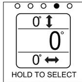
**Display Screen 5** displays the total slope angle in degrees, along with independent front-to-back angle and side-to-side angle with position indicators.
