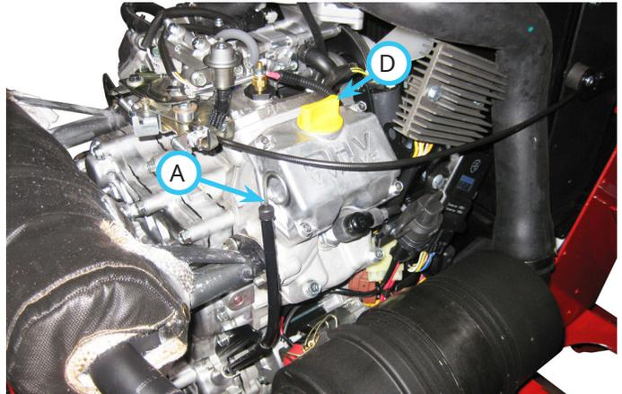
3. Insert the dipstick back into the engine and remove again.
