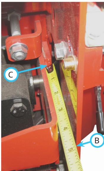
less than the measurement taken when the SDLA lever was at the neutral position. (e.g., if the original measurement was 101.6 mm (4 inches) the measurement when the neutral switch input light turns off must be between 100.8 mm (3-31/32 inch) and 100 mm (3-15/16 inch). NOTE: it is helpful to have an assistant to take the measurements.
