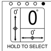
When the desired screen is reached, hold over the sensor to select and save. The slope gauge will remember the selected screen when the power unit is shut off and will display the selected screen when the power unit is restarted.
