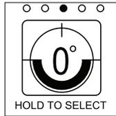
**Display Screen 4** displays the total slope angle in degrees, along with independent front-to-back angle and side-to-side angle.
