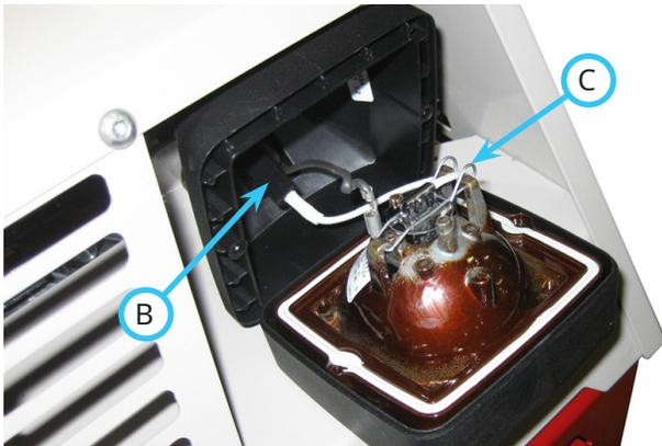
3. Pinch the wire spring fastener (C) and lift it away from the light bulb.
