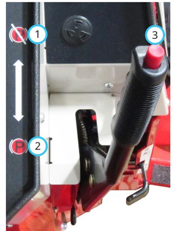
1. Parking Brake Disengaged
