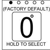
**Display Screen 2** displays the total slope angle in degrees, along with the percentage of slope.
