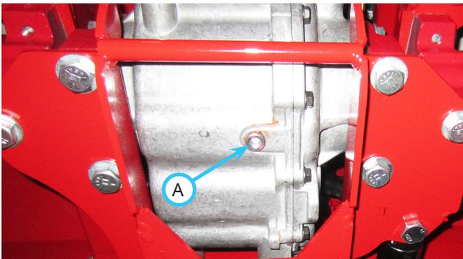
7. If the transaxle is equipped with a pipe plug, clean the drain plug and apply pipe sealant to the threads, making sure to leave the last two threads bare to prevent the thread sealant from contami-
