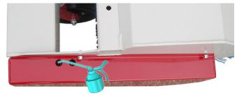
Gearbox oil level should be high enough to see in the fill tube elbow (A) when broom is parked on a level surface. Add 80-90 weight gear oil as necessary.
