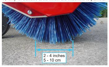
Some situations may require a more or less aggressive sweeping action. Gauge wheel adjustment, broom speed, and travel speeds are factors to apply.
