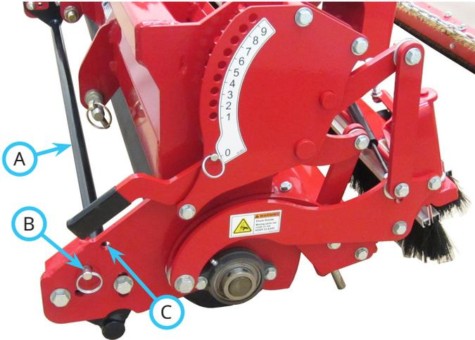
To lock the leveling bar in place, insert two pins (B) through the frame and the leveling bar end plates. To allow the leveling bar to float, remove the two pins from the frame and leveling bar end plates and place them in the storage holes (C).
