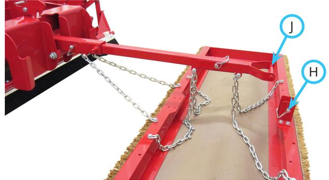
2. Lift the handle (J) up until the arm latches on the drag hitch frame.
