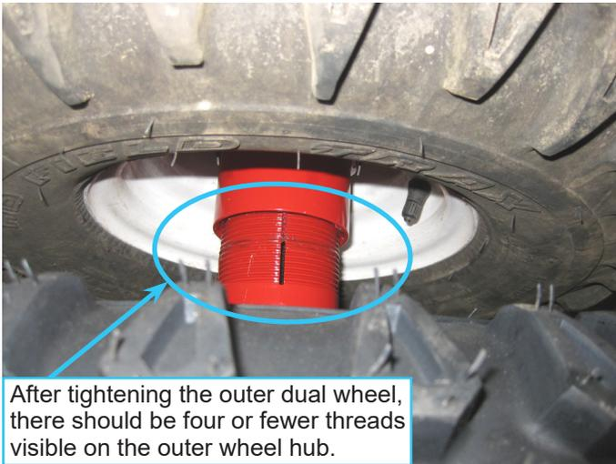
5. Tighten the draw bolt and torque to 120 ft-lbs (163 Nm). Repeat for the other three wheels.
