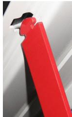
To release, move the seat prop plate over into the wide portion of the seat slot and tilt the seat forward. Lower the seat prop plate back into the seat box and lower the seat back down to the operating position.
