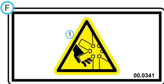
1. Cutting/dismemberment/entanglement hazard - Stay away from moving parts.
