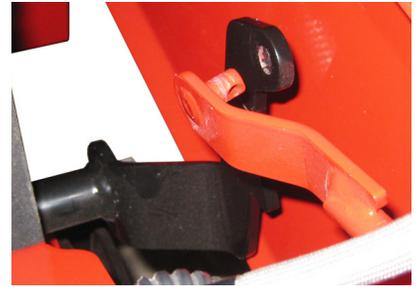
9. Lift up on the PTO idler pulley and remove the belt from the pulley.
