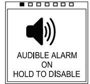
**Screen 2** changes the audible alarm set-point. Hold over the sensor until the set-point angle begins to flash. Swipe up across the sensor to cycle through the set-point options.
