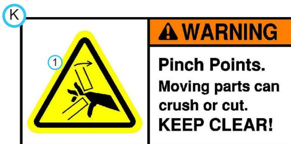
1. Cutting/crushing hazard - Stay away from moving parts.
