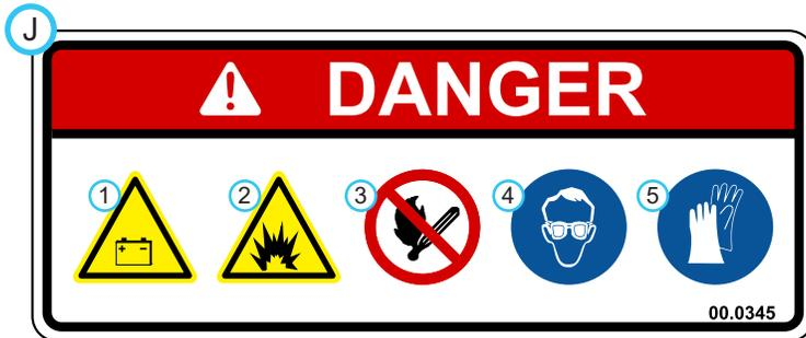
1. Danger: Battery acid is caustic and can cause chemical burns. Keep bystanders away from the battery.
