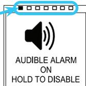
**Screen 1** allows the user to mute or enable the audible alarm. The screen will display the current state of the alarm. Hold over the sensor for 3 seconds to change the setting.
