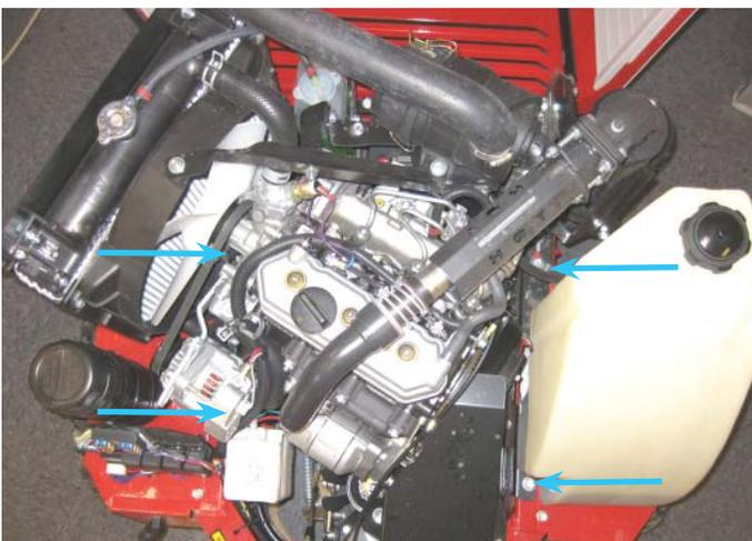
7. With bolts loosened, adjust cradle using long bolt in the back left corner of the rear frame. Adjust so that indicator bracket and end of bolt are in line (K).
