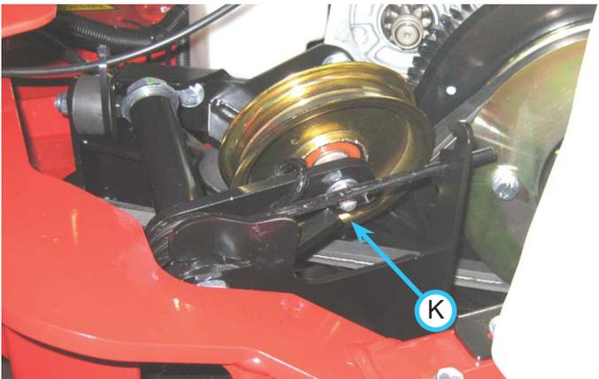
6. If position of the bolt and indicator bracket are not in-line, then the position of the engine cradle will need adjusted. To adjust the engine cradle position, loosen the four engine cradle bolts as shown at the locations shown below.
