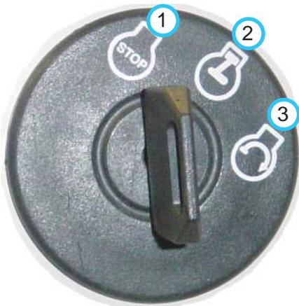
1. Off or Stop Position - All 12 volt power going through the key switch is off.
