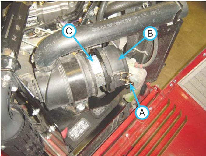
7. Remove the air filter cover (B).
