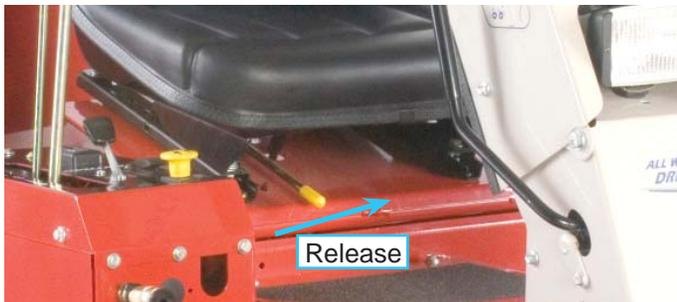
Move lever to the left to release lock. Slide the seat to the desired location and release the lever.
