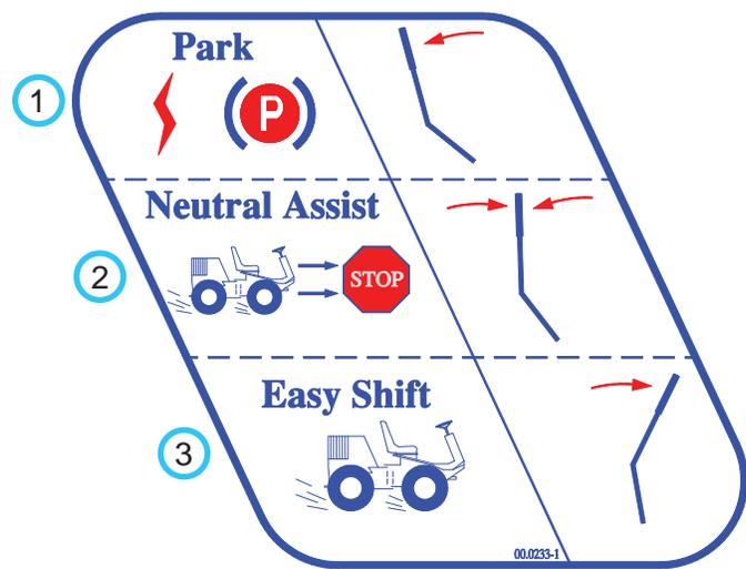
1 - In this position, the park brake is applied. The lever must be in this position for starting. When leaving the seat with the engine running, the lever must be in this position or the power unit will automatically shut off. The foot pedal control and the S.D.L.A. control lever are locked while in this position.
