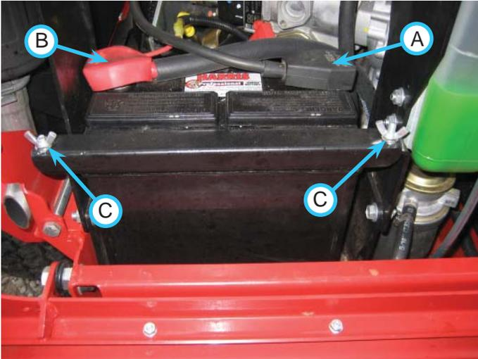
7. Loosen two fasteners (C) and remove the battery clamp.
