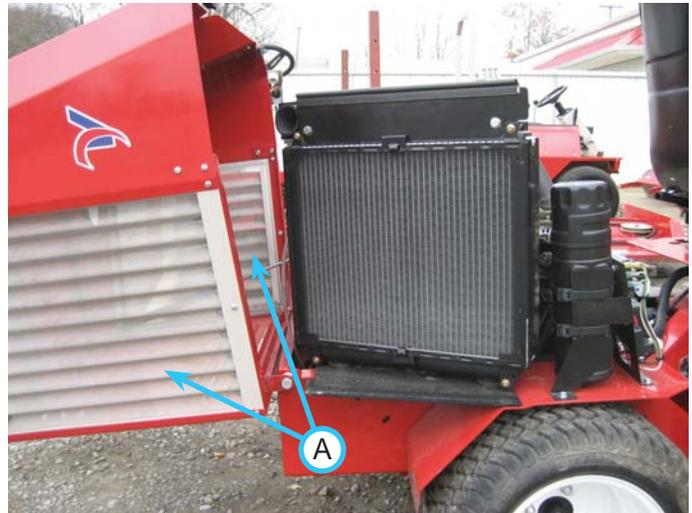
6. Clean all debris from outer screens (A) around the hood with a brush, compressed air, or water. NOTE: be sure to blow or spray from the inside out.
