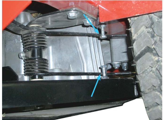
8. Slip the belt off the front double idler pulley, and then remove the belt from the PTO clutch.
