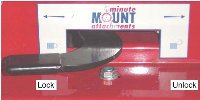
The attachment lock lever engages the hitch lock for attaching or detaching Ventrac attachments.
