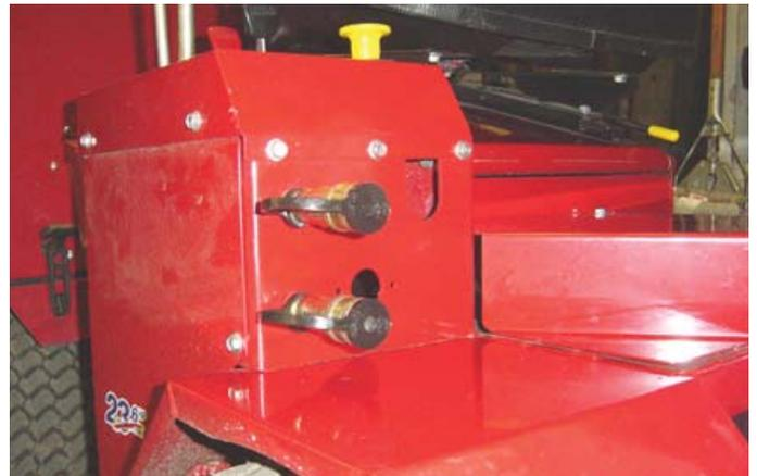
The two couplers are a part of the auxiliary hydraulic circuit and are used with an attachment which requires hydraulics (e.g. to angle a dozer blade or rotate the discharge on the snow blower).
