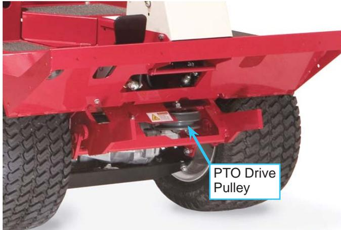
If the attachment requires a drive belt, then release the tension from the attachment drive belt and loop the belt around the drive pulley at the location shown in the figure above. When belt is in place around the bottom drive pulley, tension the belt of the attachment.
