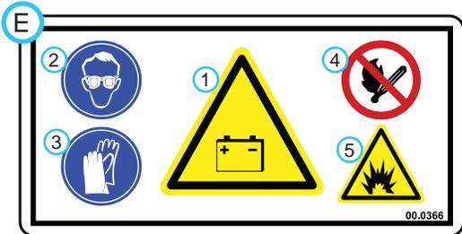
1. DANGER: Battery acid is caustic and can cause chemical burns. Keep bystanders a safe distance from the battery.
