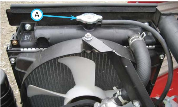
slightly and continue to turn counterclockwise and remove cap from radiator. Check that the coolant level is up to the bottom of the filler neck.
