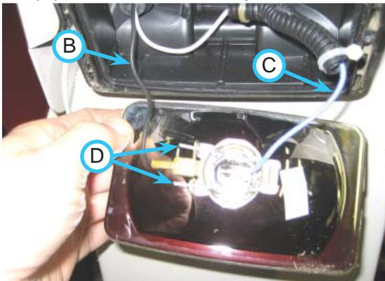
7. Remove the defective headlight from the light assembly by pinching the wire spring fastener (D).
