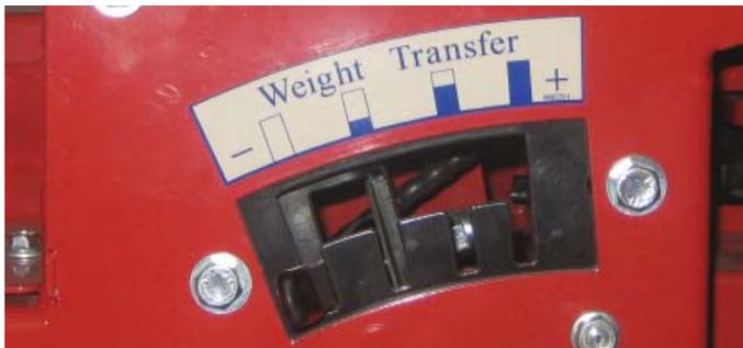
The weight transfer system transfers weight from the attachment to the front wheels of the power unit. The operator can select different transfer rates by selecting one of the four positions. Note: the front hitch must be fully raised to adjust the lever.
