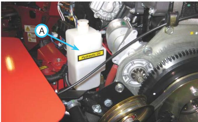
6. Visually inspect to see that the level of hydraulic oil is centered between the low and full marks of the tank. Note: use a flashlight to inspect level if necessary.
