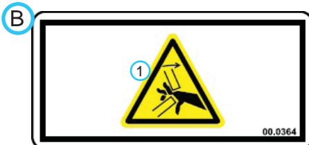
1. WARNING: Cutting/crushing hazard - Stay away from moving parts.
