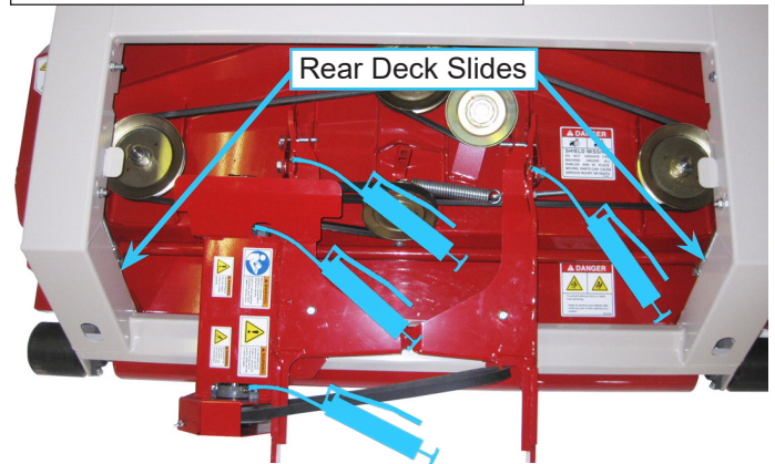
Hitch Pivots, Drive Shaft Bearings, & Rear Deck Slides
