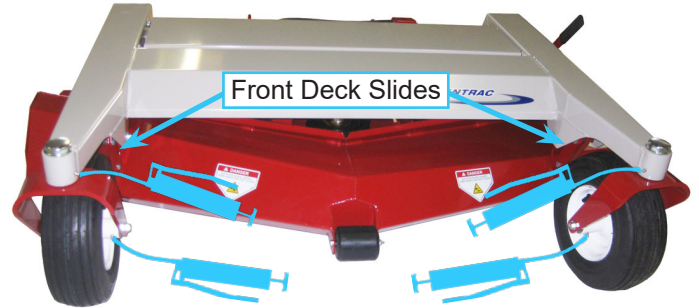
Caster Wheel Pivot, Wheel Axle Bearings, & Front Deck Slides
