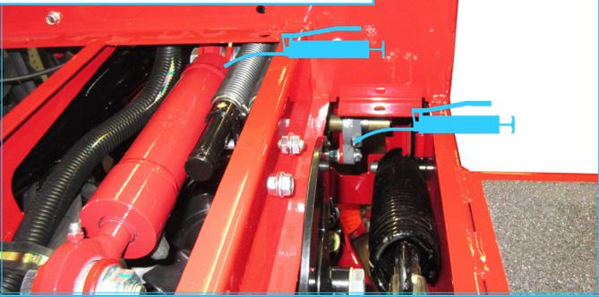
The rear grease fitting on the lift cylinder must be greased from below the cylinder by removing the weight transfer access cover and using a grease gun with a flexible hose.
