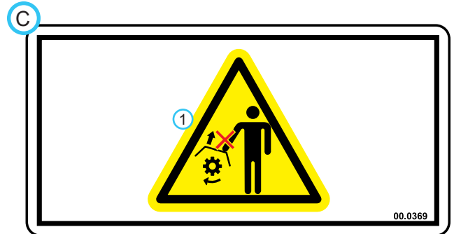
1. Cutting / dismemberment / entanglement hazard - Do not remove shields. Stay away from moving parts.
