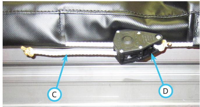
After placing the hopper cover over the hopper, pull out on the cord (C) to cinch the cover in place. Push in on the ratchet latch (D) to release the cord and remove the cover.
