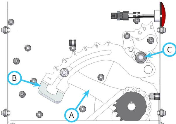
The gate control rocker mounting bolts (C) can be adjusted to increase or decrease the overall opening of the gate.
