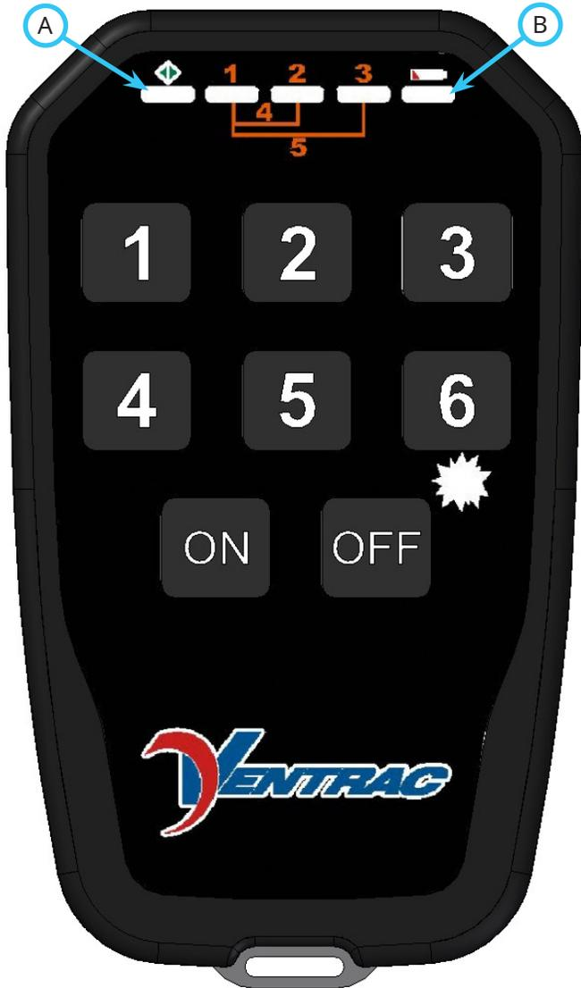
Press and hold the On button until the power on indicator (A) flashes (approximately 1 second) to turn on the control unit.
