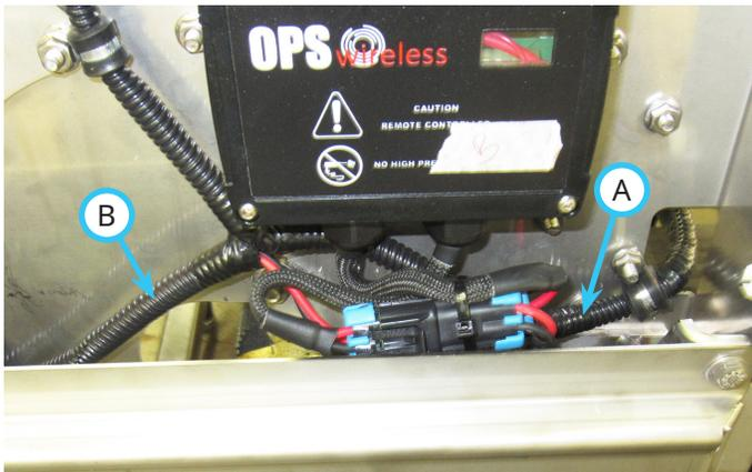
4. Unplug the motor harness (B) from the controller unit connector and plug the motor wire harness connector and the power supply wire harness connector together.
