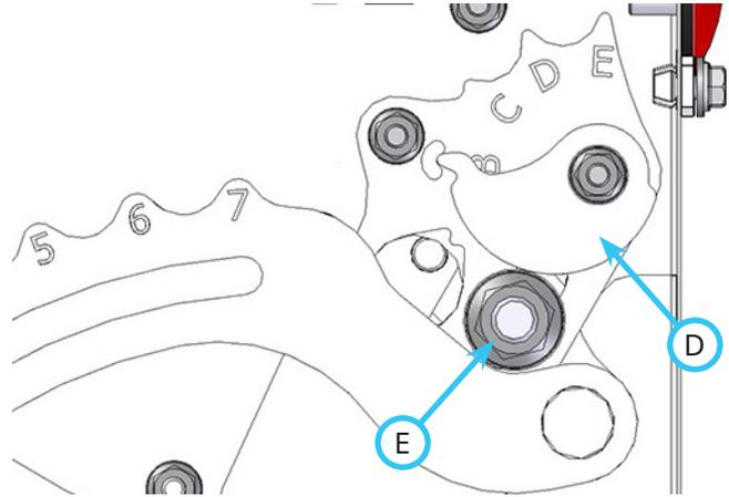
3. Loosen the nuts (E) that fasten the gate control rocker to the end panels and the stiffener plates.
