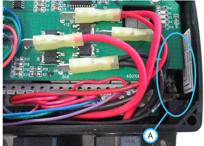
5. Remove one of the two jumpers from the jumper rest positions and install it in the pairing position. Refer to the label inside controller housing.
