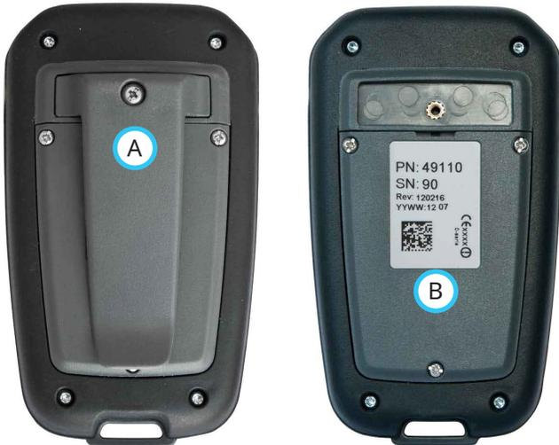
2. Remove the three screws that fasten the battery compartment cover (B) to the remote control.
