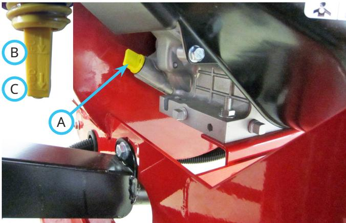
3. Check the oil level. The oil level should be between the Full (B) and Add (C) marks on the dipstick.
