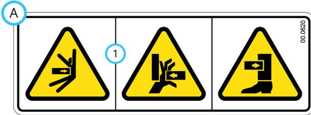
1. Pinching or crushing hazard.
