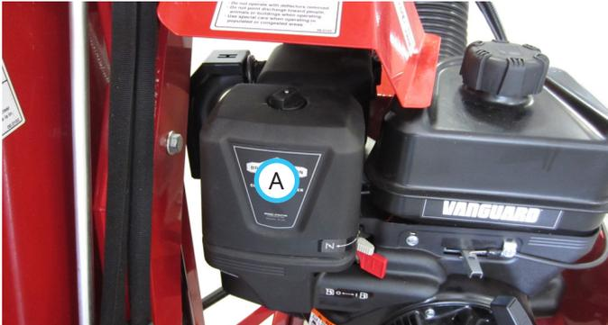
3. Remove the foam pre-cleaner from the air filter element.
