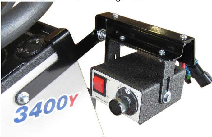
29. Connect the battery/controller harness to the battery lead on the controller.
