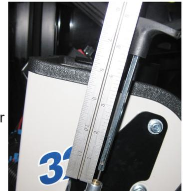
28. Cut the cable to length at the marked location and then push the cable handle back into the housing.
