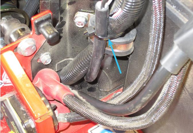
38. Coil up any excess wire in the rear frame and use zip ties to fasten to the rear hitch support on the rear frame.
