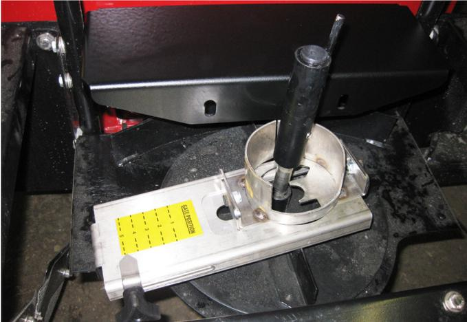
24. Place the plastic hopper throat into the gate assembly and temporarily install a cushioned metal clamp to both of the outer hopper mounting holes. Do not tighten as these will be removed again. Route the gate cable through the two clamps.
