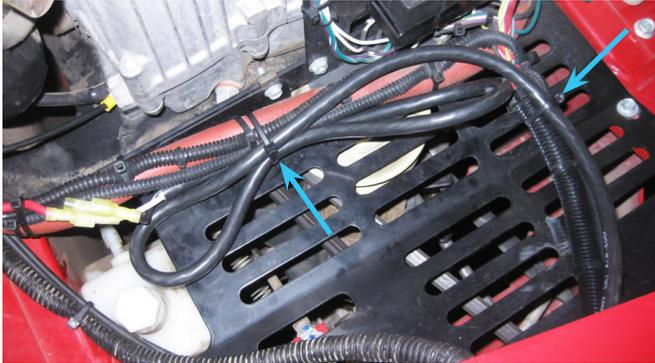
9. Install the circuit breaker into the fuse holder on the positive wire harness.
