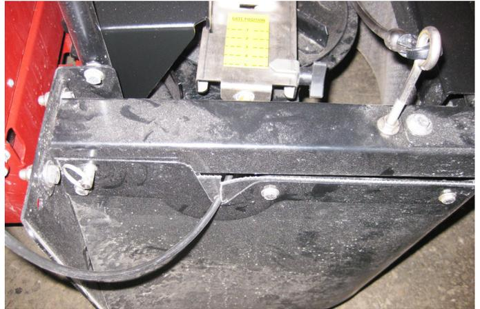
34. Install the plastic hopper throat into the gate assembly. It will probably be necessary to trim off the hopper throat so the mounting holes line up with the frame holes. To determine the amount to trim, make sure the hopper throat is bottomed out in the gate assembly, then measure the distance the bolt holes in the hopper need to move to line up with the spreader frame holes. Add 1/16" (2 mm) to this measurement and cut the hopper throat back that amount.
