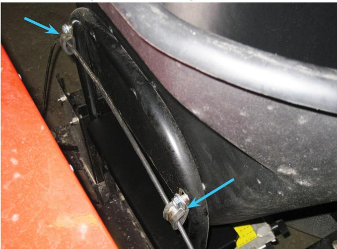
25. Determine how long the cable should be by holding it up to the gate assembly. Make sure there is enough slack in the cable to allow the spreader to swing out so the power unit hood can be opened. Also make sure there is a large enough loop at the spreader that a curtain kit will work if one is installed.
