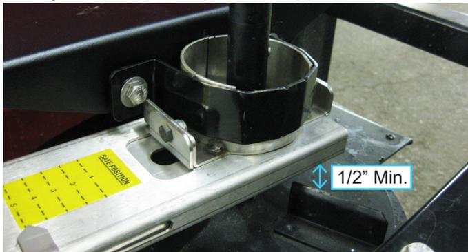
Move the hopper throat clamp in the gate mount slots until there is a minimum of 1/2" (12.7 mm) clearance between the spinner and the bottom of the gate assembly.
