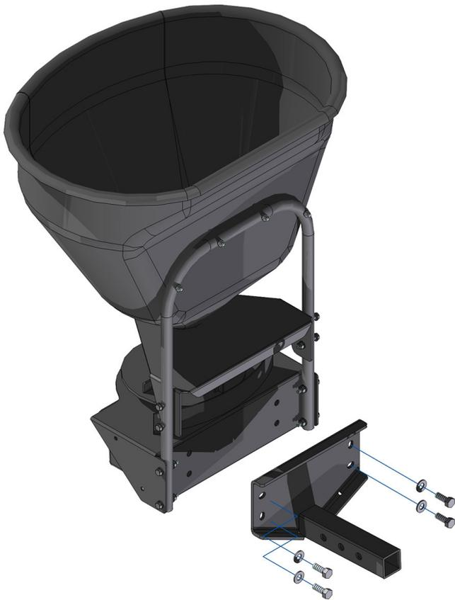
2. Slide the spreader hitch tube into the hitch receiver and fasten with the included 5/8 x 3" hitch pin. Use the hole in the spreader hitch tube that positions the spreader closest to the power unit without any contact between them.
