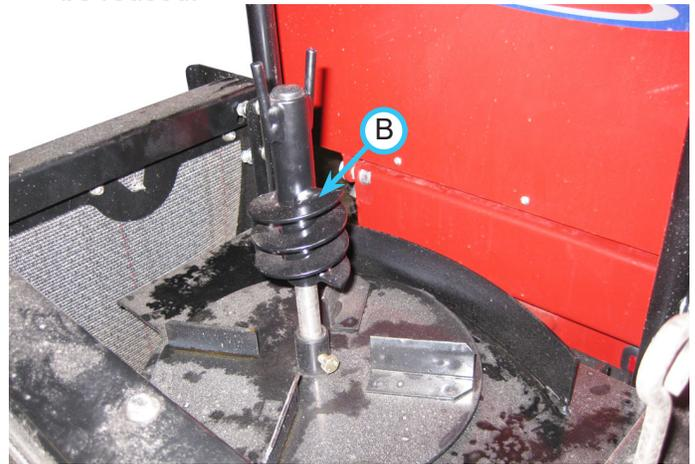
6. Remove the 4) bolts that fasten the hopper support plate (A) to the tube frame and remove the hopper support plate. The plate will not be reused.
