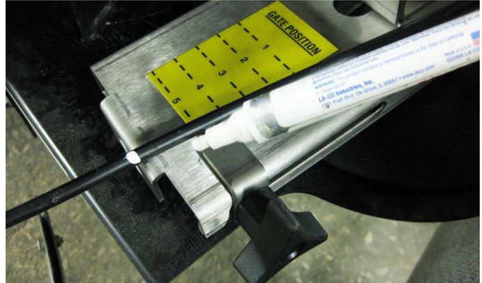
27. Pull the cable handle up until there is approximately 5" (12.5 cm) between the bottom of the cable knob and the top nut that fastens the cable to the gate cable mount. This will ensure that when the cable is cut to length, that there will be enough length of inner cable wire to connect to the gate slide.
