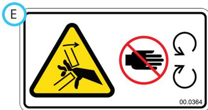
Pinching or crushing hazard.
