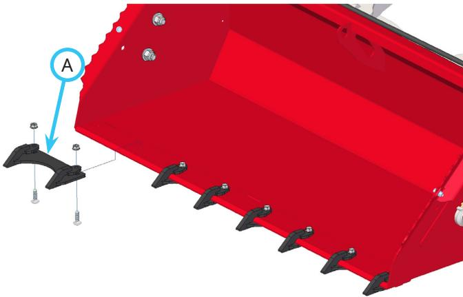
5. Secure each set of teeth to the power bucket using two 3/8 x 1-1/4 inch carriage bolts inserted up through the tooth and bucket. Secure with two flange nuts and torque to 42 Nm (31 ft-lb).
