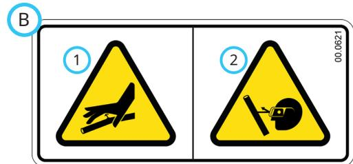
1. High pressure fluid hazard - keep your body and hands away from suspected hydraulic leaks.
