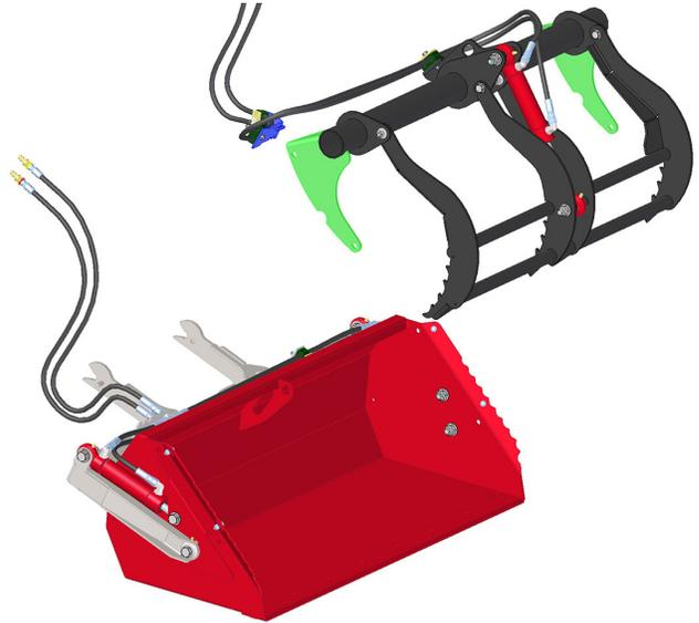
3. Install two 1/2 x 1-1/2 inch carriage bolts through both the right and left grapple frame brackets and the bucket sides and fasten with 1/2 inch nylon locking flange nuts. Torque to 102 Nm (75 ft-lb).
