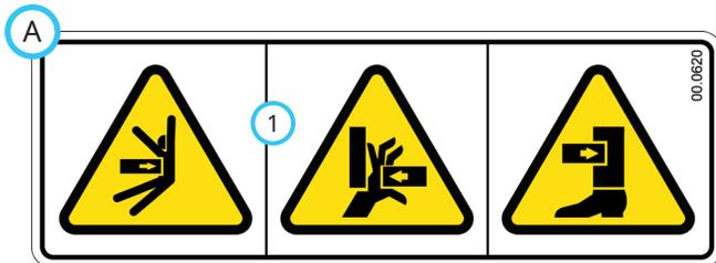
1. Pinching or crushing hazard.
