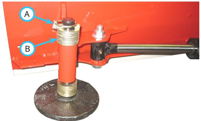
4. Remove the skid shoe from the bottom of the skid shoe mount. Add or remove spacer washers to reach the desired skid shoe height and insert the skid shoe into the skid shoe mount. Place any extra spacer washers on top of the skid shoe mount and fasten the skid shoe in place with the lynch pin. Both the right and left skid shoes should be set at the same height.
