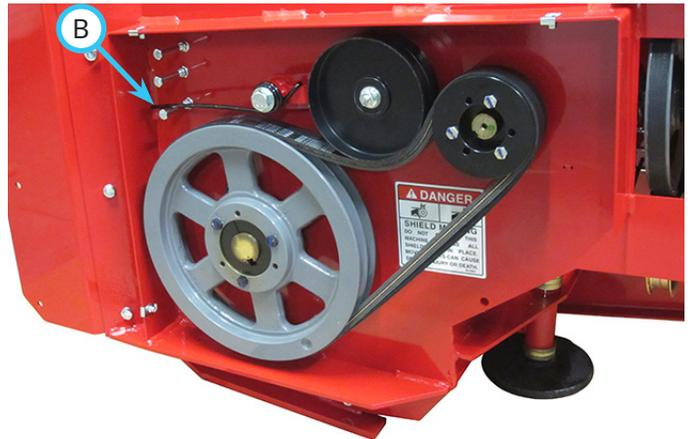
3. Remove the old auger drive belts and install the new drive belts onto the pulleys.
