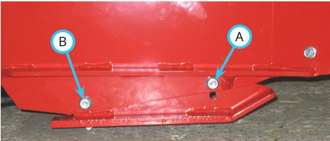
4. If the front of the skid shoe needs to be lowered, remove the front mounting bolt (A), lower the front of the skid shoe, and reinstall the bolt. The rear of the skid shoe is slotted so the skid shoe can be rotated down without removing the bolt.
