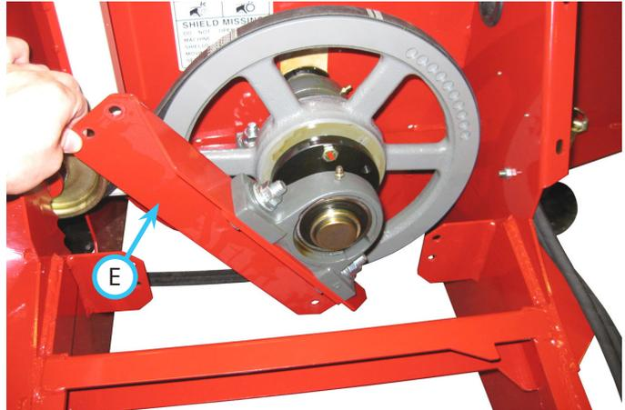
6. Remove the old fan drive belt from the pulleys and remove through the opening between the fan shaft bearing mount and the snow blower frame.
