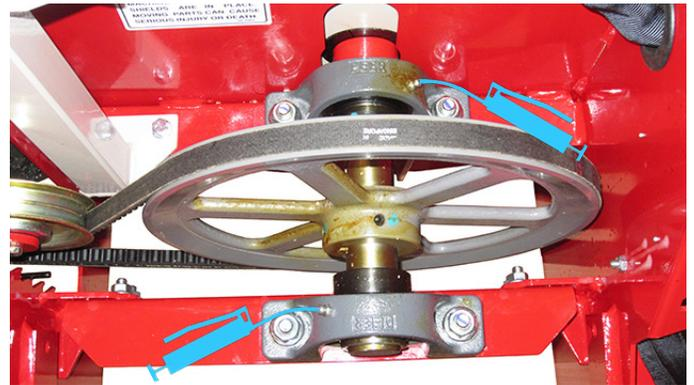
3. Grease the drive shaft bearings.
