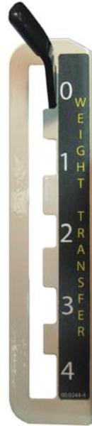
0 – Off. This position does not transfer any weight from the attachment to the tractor.
