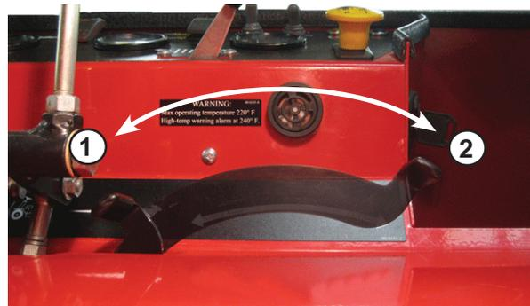
1 - S.D.L.A. control lever has a “spring assist to neutral” action. When removing your hand from the S.D.L.A. control lever it will automatically return to neutral. This position makes neutral easy to find and maintain. It is recommended that this position be used when learning the operation of the Ventrac, loading & unloading, attaching and removing attachments and whenever the operator is working in tight areas or unsure of the machines response to the task being performed.
