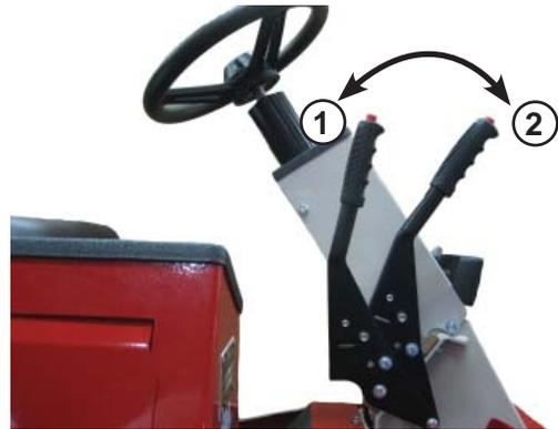
1. Park & Emergency position: The lever must be in this position for starting the machine, and when leaving the seat with the engine running. Foot pedal control and the S.D.L.A. control lever are also locked while in this position.
