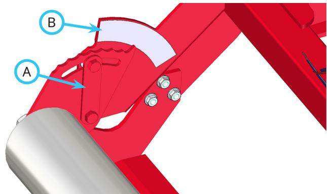
2. Rotate the roller until the depth indicator points to the desired depth on the height adjustment decal (B).
