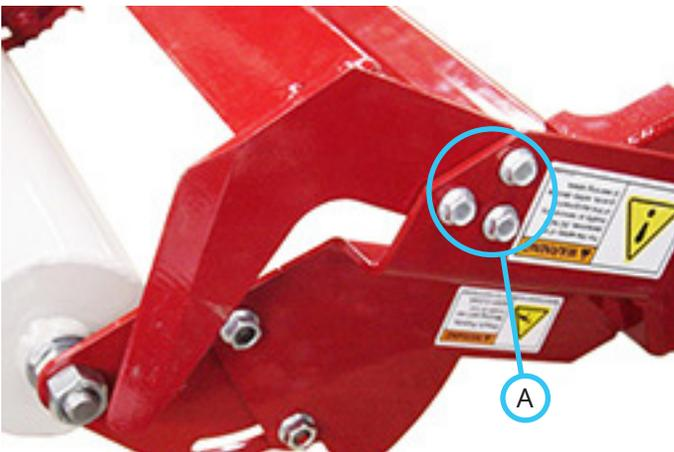
3. Remove the old cutting blade and position the new cutting blade in place.
