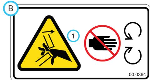
1. Cutting or pinching hazard. Stay away from moving parts.
