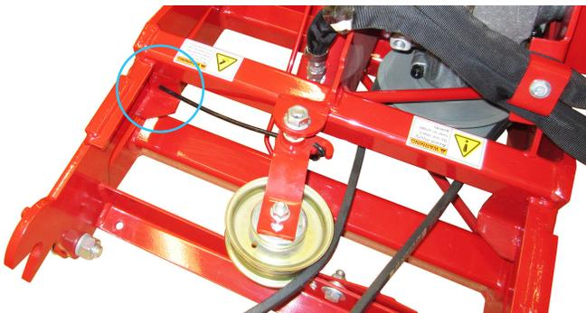
6. Ensure the drive belt is properly located in the pulley grooves before attempting to operate.
