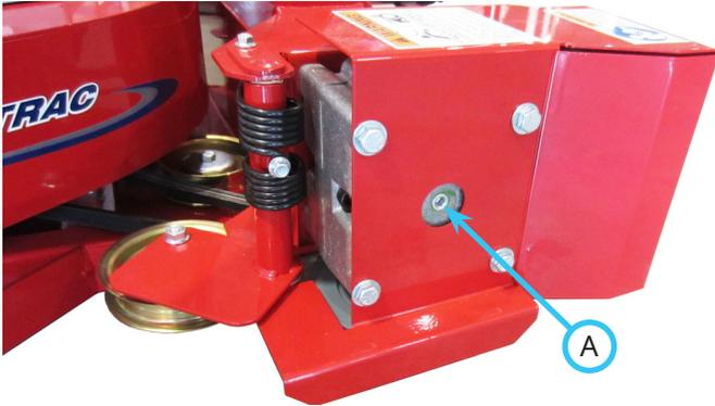
3. Use a fluid extractor to remove the old gear oil from the gearbox.
