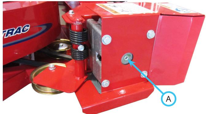
3. Check the oil level in the gearbox. The oil level should be maintained at the bottom of the fill hole. If the oil level is low, add 80-90 synthetic gear oil until the oil level reaches the bottom of the fill hole.
