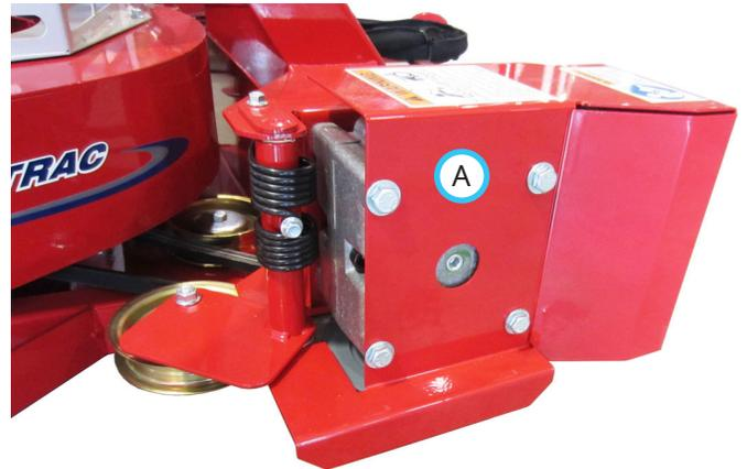
3. Remove the old drive belt and place the new drive belt onto the pulley.
