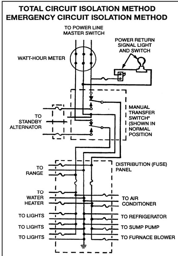
\*Ampere rating must equal or exceed the ampere rating of the incoming utility service.
