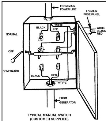
\* MANUAL TRANSFER SWITCH POSITION DETERMINES WHICH POWER SOURCE, UTILITY OR STANDBY GENERATOR WILL FEED INTO THE DISTRIBUTION PANEL
