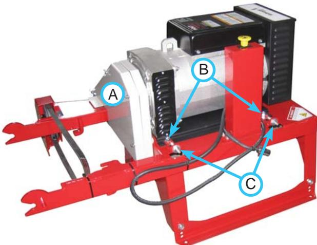
1. If the generator drive belt requires tension adjustment, detach the generator from the power unit.
