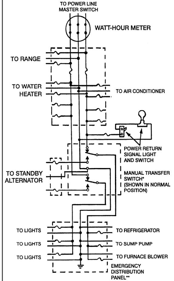
\*Ampere rating must equal or exceed the ampere rating of the emergency distribution panel.
