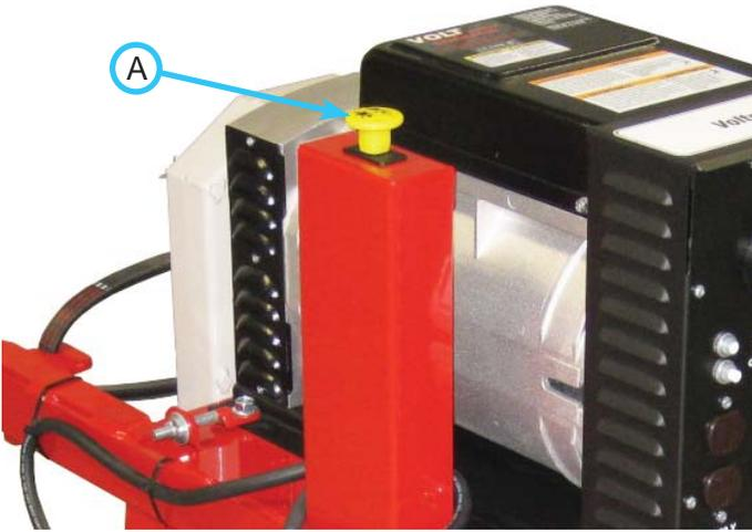
The remote PTO switch (A) allows the power unit's PTO\* to be shut off from the generator. The power unit must be equipped with an electric PTO remote (kit # 70.4078) in order for the generator's remote PTO switch to be used.
