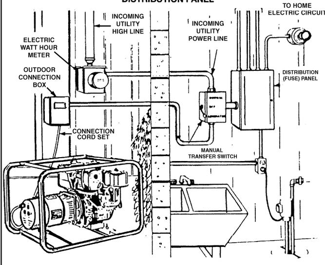
This generator does not have output capacity to power your entire home. Most home utility commercial electric service is in excess of 100 amperes at 240 volts, which exceeds the output of the generator. Because of this, only key items can be powered (up to the ampere rating of the generator) during a commercial power outage. There are two methods of installing a manual transfer switch, the emergency circuit isolation method and the total circuit isolation method.
