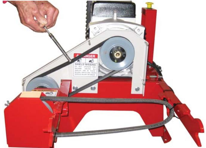
5. If the belt tension does not fall in this range, adjust the belt tension by tightening the nuts on the generator belt adjusters (C) to apply more belt tension or loosening the nuts on the generator belt adjusters to lessen the belt tension.
