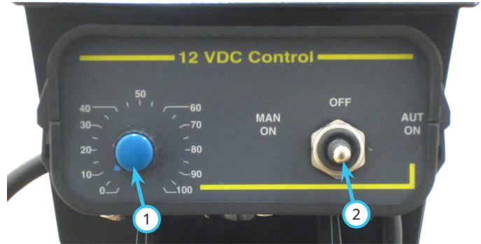
Power is sent to the motor by moving the switch to either MAN ON or AUT ON. Moving the switch to the MAN ON position disregards the speed control dial and sends full power to the motor. Moving the switch to AUT ON allows the motor speed to be controlled by the speed control dial setting.
