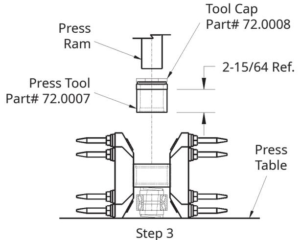
3. Press the used bearing and adapter assembly out of the rotor.
