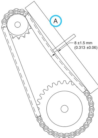
5. If the chain tension needs adjusted, proceed to the following section for chain tension adjustment. If the chain tension is correct, reinstall the motor cover and torque the bolts to 11 Nm (100 in-lbs).
