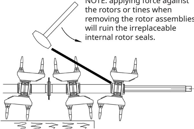
4. Clean and inspect the parts as they are removed and set aside in their order of removal.
