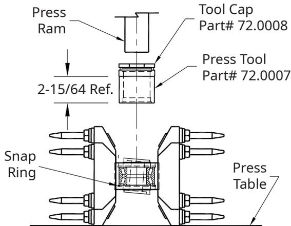
3. Install a snap ring in the other end of the rotor hub.
