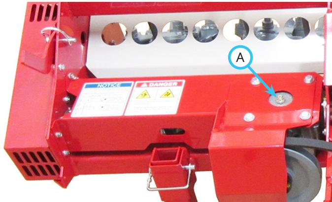
2. Check the oil level in the gearbox. The oil level should be maintained at approximately half full. If the oil level is low, add 80-90 synthetic gear oil until the proper level is reached.
