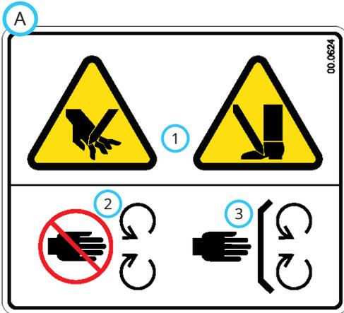
1. Cutting or puncture hazard - hand or foot.
