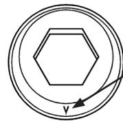
2. Use a marker pen to assist with aligning timing marks between rotors. Mark two rotor shaft flats 180 degrees apart next to the threaded end. The marked flats must align with the timing marks of any rotors not removed during servicing.
