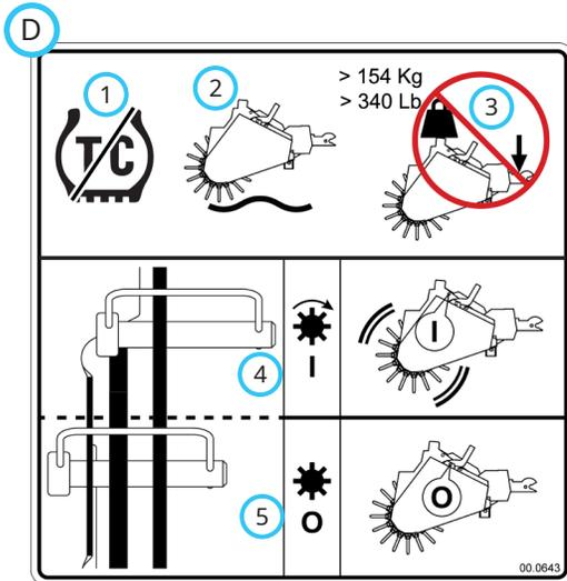
1. Turn off the power unit's weight transfer system.
