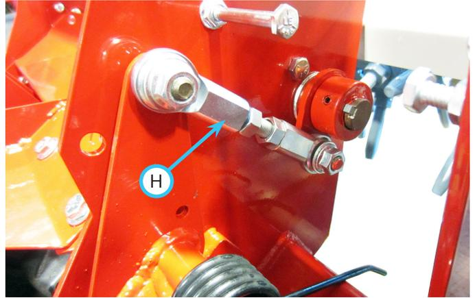
NOTE: shorten the clutch linkage (H) to move the clutch pulley (F) down toward the belt. Lengthen the clutch linkage to move the clutch pulley up away from the belts.
