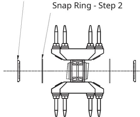
2. Remove the snap rings on both sides of the rotor.
